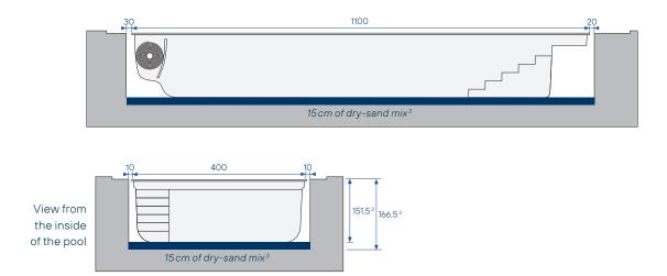
Note: the digging sizes do not take into account the necessary space for the coping stones. <sup>1</sup> Needed for unloading & placing the pool. <sup>2</sup> Depth taken from under the coping stone. <sup>3</sup> Mix of sand and cement, at a ratio of 250 kg per ton.
