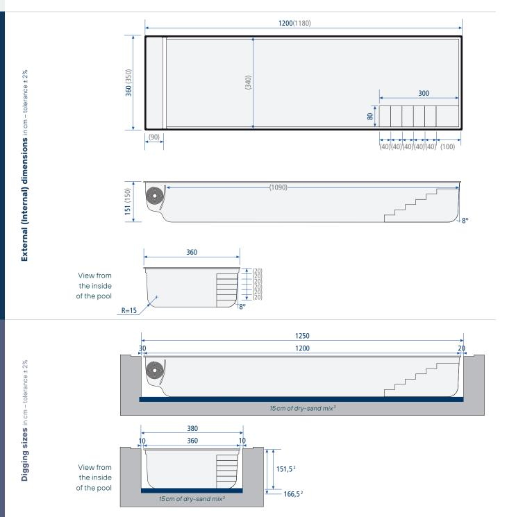
Note: the digging sizes do not take into account the necessary space for the coping stones.
