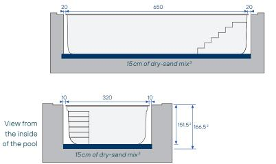
Note: the digging sizes do not take into account the necessary space for the coping stones.
